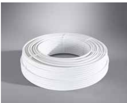
KLIMAPEX® metal composite pipe PE-RT/AL/PE-RT 16 x 2.0 made of polyethylene with welded aluminium jacket, multi-layer composite pipe, diffusion-tight and dimensionally stable
